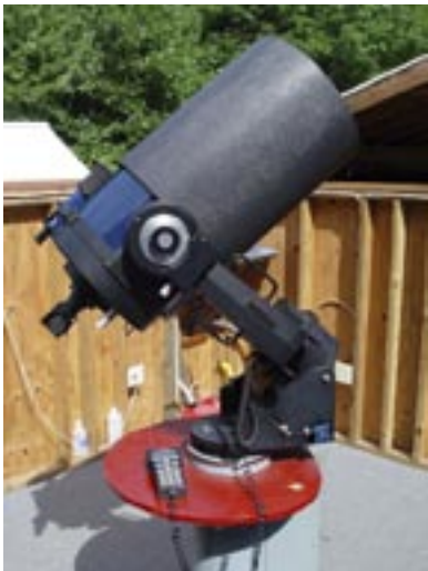
The 12-inch Meade LX200 Schmidt-Cassegrain telescope. Photo by Jim Crawford.
