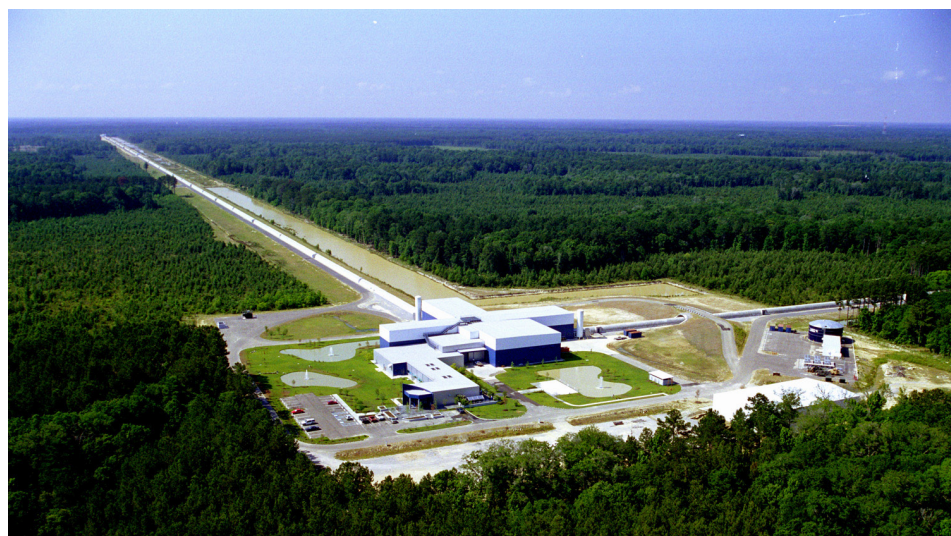
Laser Interferometer Gravitational-wave Observatory in Livingston, Louisiana. Each of the two arms is 4 kilometers long. LIGO has another such observatory in Hanford, Washington.
