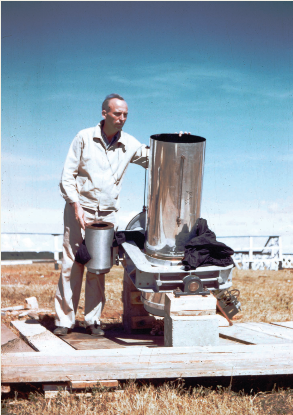
Smiley with 4-inch f/1 Schmidt camera and 12-inch F/3.5 Schwarzschild camera at eclipse site in Araxa Brazil for May 20, 1947 total solar eclipse - which was clouded out.
