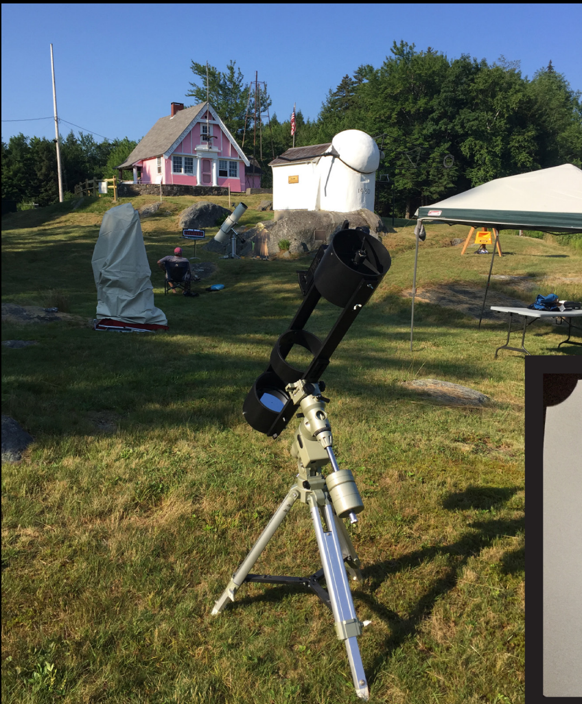
On Wednesday, July 19, the eve of the 2017 Stellafane Convention, Bob Horton brought his newly completed 6" f/6.5 Newtonian telescope to Seagrave Observatory to collimate and evaluate it before entering it in the optical competition. Francine Jackson and Jim Hendrickson were also in attendance. The telescope performed exceptionally well under the hazy skies, providing great view of Saturn and Epsilon Lyrae.
