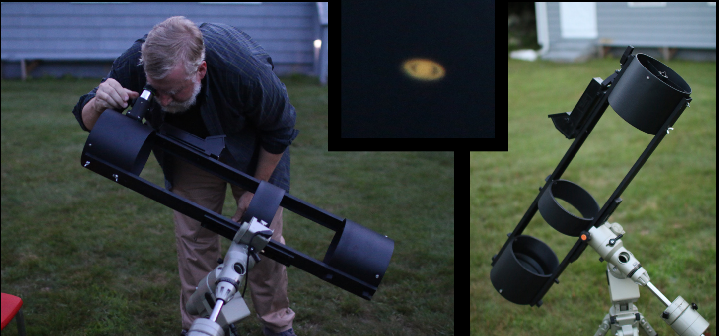
On Wednesday, July 19, the eve of the 2017 Stellafane Convention, Bob Horton brought his newly completed 6" f/6.5 Newtonian telescope to Seagrave Observatory to collimate and evaluate it before entering it in the optical competition. Francine Jackson and Jim Hendrickson were also in attendance. The telescope performed exceptionally well under the hazy skies, providing great view of Saturn and Epsilon Lyrae.
