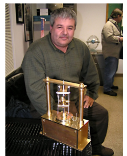
The Alvan Clark refractor in late 2006. Al Hall is rebuilding the flyball governor to replace the electric motor that drives the telescope.
