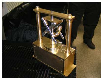
The Alvan Clark refractor in late 2006. Al Hall is rebuilding the flyball governor to replace the electric motor that drives the telescope.
