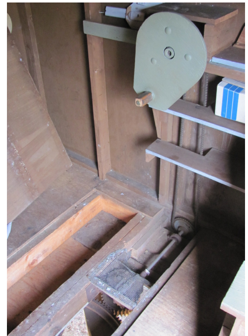
L) The sliding door and roof panel in place. R) the crank and chain apparatus connected to the under-floor gear system
