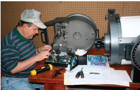
Top: Bob Horton and Jim Brenek disassemble the 16" Meade. Bottom: Bob Napier tests the electronics to determine the source of a problem with the drive system. Photos by Chris Chapman.
