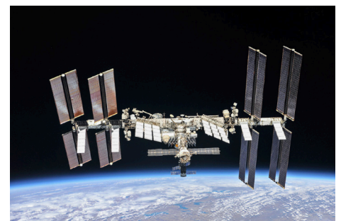
A complete view of the ISS as of October 4, 2018, taken from the Soyuz capsule of the departing crew of Expedition 56 from their Soyuz capsule. This structure was built by materials launched into orbit by 37 United States Space Shuttle missions and 5 Russian Proton and Soyuz rockets, and assembled and maintained by 230 spacewalks, with more to come! Credit: NASA/Roscosmos More info: bit.ly/issbasics
