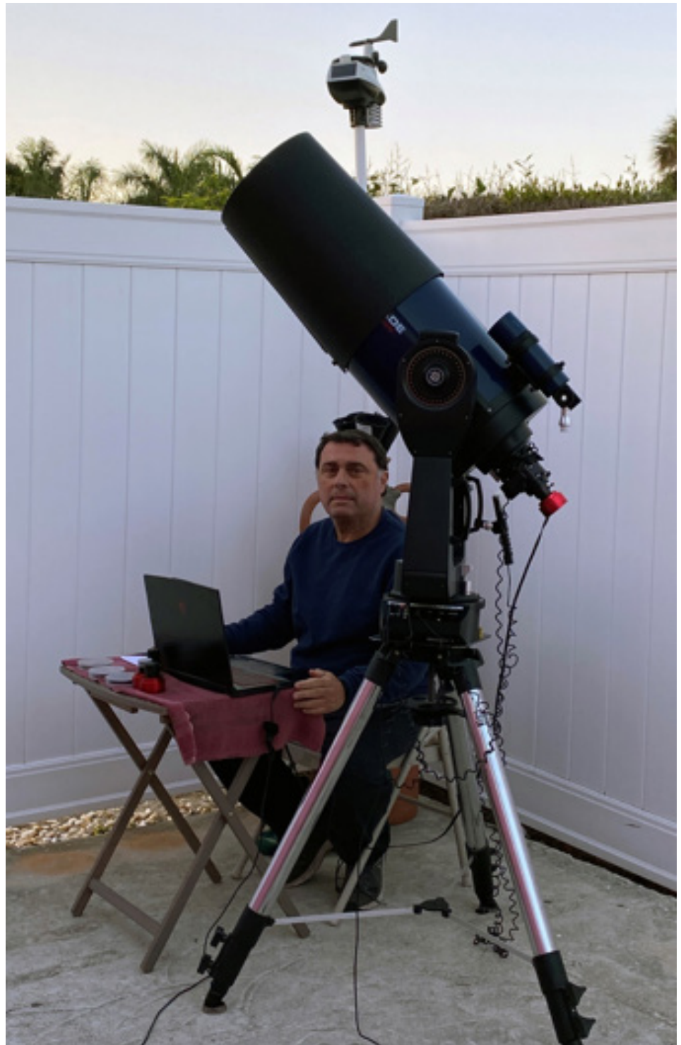
Figure 4: The author with his 10-inch Meade LX200GPS Schmidt-Cassegrain telescope, ZWO cameras, assortment of filters and MSI GF65 six core 12 thread upgraded to 40GB RAM gaming computer. He recommends using a high-end gaming laptop to greatly reduce video processing time because they use high-end graphic cards, processors and RAM. A fenced in area also helps shield the area from unexpected wind gusts. Part of an Ambient Weather WS8480 weather station can also be seen at the top center of photo. (Photo courtesy of the author).
