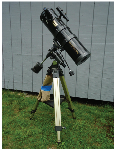
Orion SkyView 6-inch Reflector on Equatorial Mount
