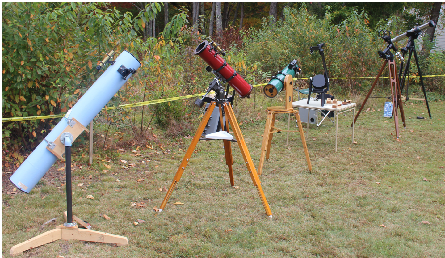
Home-made telescopes on display: John Leonelli's 6" f/8, Bob Horton's 4.25" f/6.3, Glenn Jackson's 6" f/5, Jim Brenek's 8" f/4.8 & equatorial mount, and Dick Parker's 4" f/10 achromat doublet.
