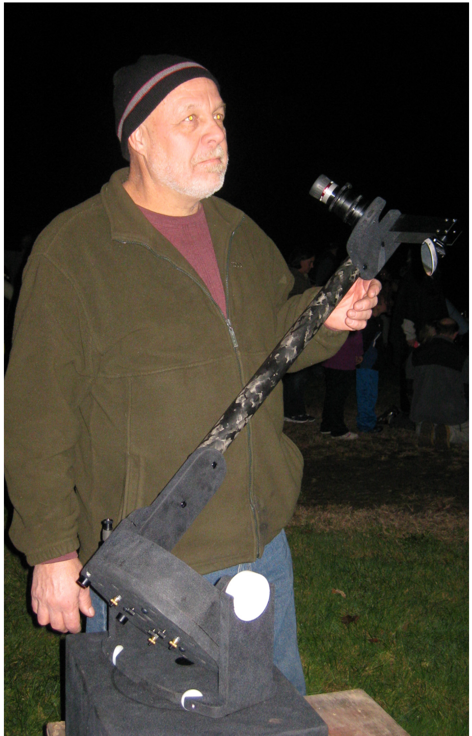
Jim Brenek set up his newly completed 8-inch f/4.5 telescope at the Callahan School star party on October 22. The telescope includes a custom secondary support and focuser. Jim made the telescope with birch plywood, carbon fiber and aluminum. The Pyrex mirror was figured at Dick Parker's workshop. All wood surfaces are flocked.
