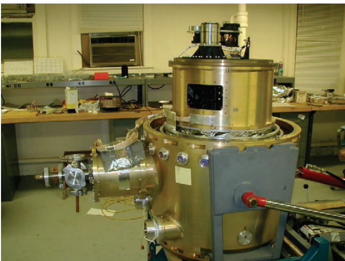
Also being constructed in the basement at Yerkes is H.A.W.C. A 2.7 meter infra-red High resolution Airborne Wide band Camera, which is being built by the University of Chicago. The HAWC will fly on the NASA S.O.F.I.A. 747 upon completion.
