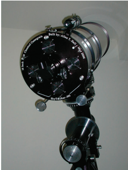
Al Hall recently completed his 16" Cassegrain telescope and its accompanying German equatorial mount, which Al and Dick Parker have been working on for several years. Al expects to have first light sometime in the next 2 weeks, then he will be taking it to Breezy Hill to enter it in the 2008 Stellafane amateur telescope making competition.
