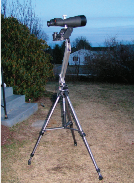
Quantaray Titan tripod with T and T Bino mount and homemade swing arm mount.
