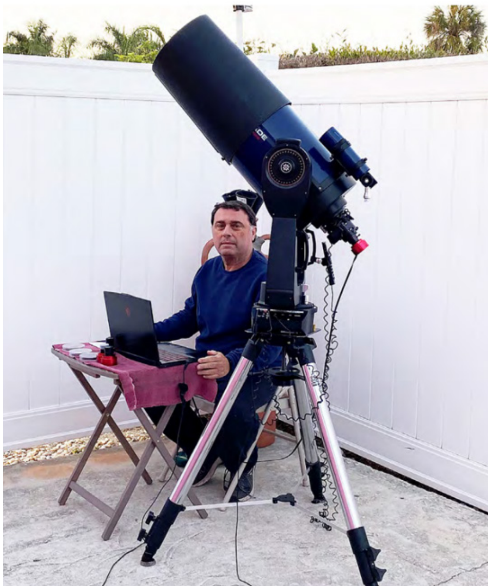
Figure 3: The author with his imaging setup. A Meade LX200GPS 10-inch 2500mm at f/10 with a ZWO ASI 462MM monochrome camera, Vernonscope 1.25x Barlow, and Baader 610nm R-IR longpass filter. An MSI GF65 i7 six-core 12-thread upgraded to 40GB of RAM gaming computer greatly reduces video processing time. Firecapture 2.7.0.15 captured the 75 second SER videos which were aligned & stacked with Autostakkert 4.0.13, sharpened and with Registax 6.1.0.8. Slight deconvolution with AstralImage 5.2.3.0 and additional processing in Photoshop CS4.
